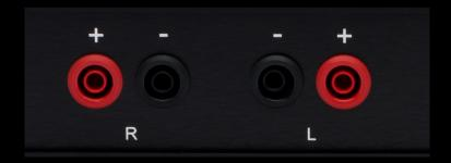
Your speaker cables will most likely have the same coloured ends so the first step is simply to match your coloured speaker cables with the speaker socket colours on the back of the amplifier which have been clearly marked Left and Right.
